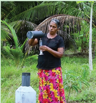
Manual rain gauge for irrigation management
